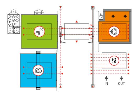
The KOMBY Multiline systems include a central overhead bridge conveyor, and a dedicated loading/unloading area. If other modules are integrated to this process, such as a pre-treatment spray tunnel, automatic powder coating booths, this equipment ensures total flexibility to work plus a quality check of the finishes.
