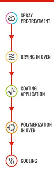
After being loaded onto the overhead conveyor, the pieces are processed inside a spray washing tunnel to undergo a chemical cycle suitable for the surface to be treated and the quality to be obtained. The cycle comprises several stages of degreasing, washing and processing with other chemical solutions.
